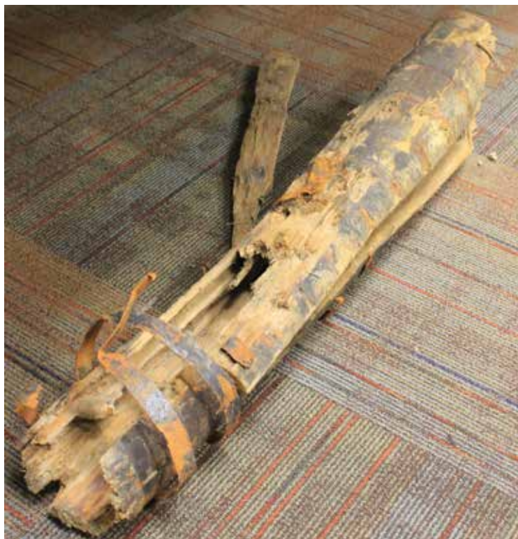
A section of wooden pipe once used in the city of Ree Heights
